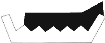
Fig. 6: Identifying Drive Belt Incorrect Installation Courtesy of FORD MOTOR CO.
