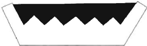
Fig. 7: Identifying Correct Installation Of Drive Belt Courtesy of FORD MOTOR CO.
